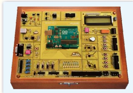
This IOT trainer is to make different types of IOT projects and learn Hardware, Sensors, programming and controlling data by Mobile - SMS or by Internet
